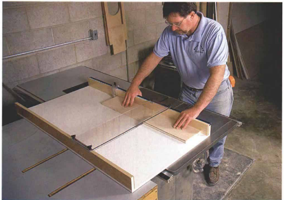
Shop sled. This shop-built jig makes crosscutting items such as cabinet components fast, safe and easy with its large capacity and pinpoint accuracy.
